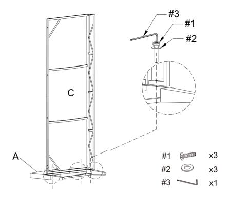
Step 2. Attach back panel (part D) to right arm panel (part A) and seat panel (part C) using bolts (part #1), flat washers (part #2) and allen wrench (part #3).
