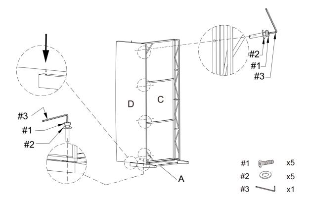
Step 3. Attach left arm panel (part B) to back panel (part D) and seat panel (part C) using bolts (part #1), flat washers (part #2) and allen wrench (part #3).
